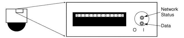
**Data LED**: This LED indicates the status of data transmission. After power is supplied, it is on for the first 4-5 seconds and then it goes off. It blinks continuously when a user accesses the VersaCam and is transmitting data.
